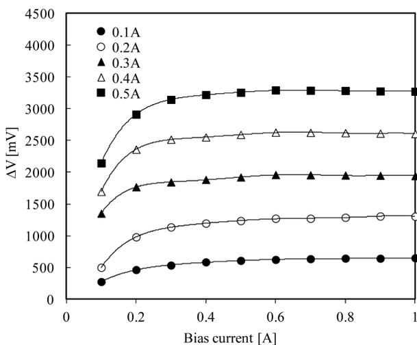
Fig. 4. Bias current dependence of voltage differences for the excitation current of 0.1, 0.2, 0.3, 0.4 and 0.5. Voltage difference  $\Delta V$  was evaluated by subtraction of the voltage measured without magnetic field from the voltage measured with the magnetic field of 15 Oe.
