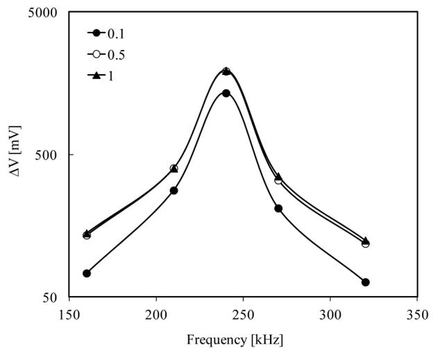
**Fig. 3.** Frequency dependence of voltage differences for the bias current of 0.1, 0.5 and 1 A. Voltage difference  $\Delta V$  was evaluated by subtraction of the voltage measured without magnetic field from the voltage measured with the magnetic field of 15 Oe.
