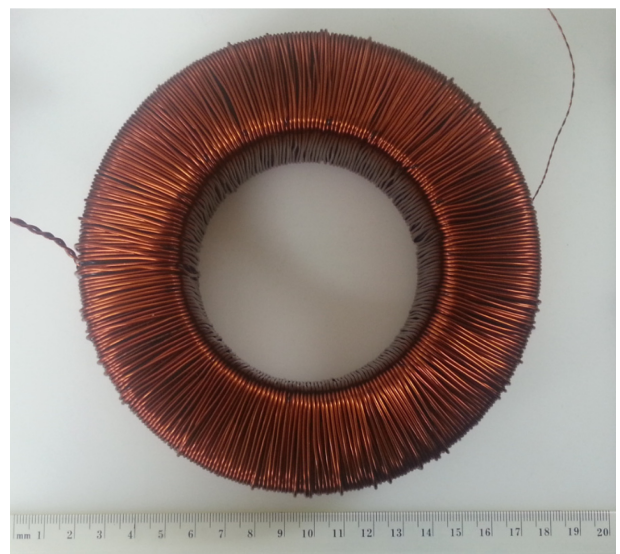
Fig. 4. (Color online) Photography of the coil wound metallic powder core; dimension of core (OD: 134 mm, ID: 77 mm, height: 42 mm), N_1 = 401 turns, N_2 = 5 turns.
