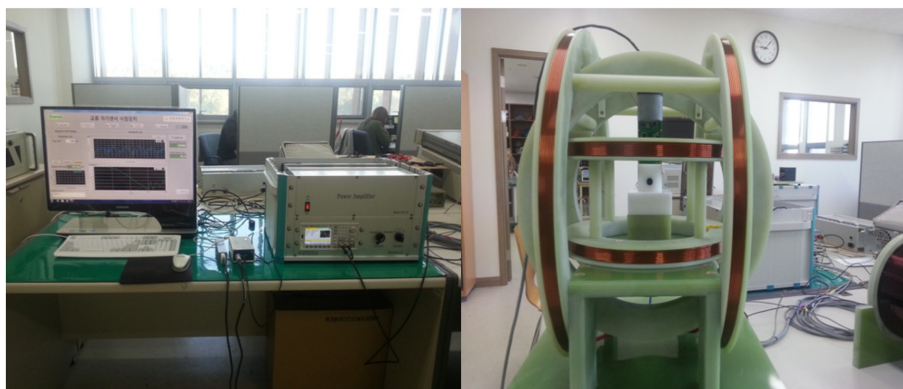
Fig. 5. (Color online) 3-axis Helmholtz coil system for the frequency bandwidth measurement.
