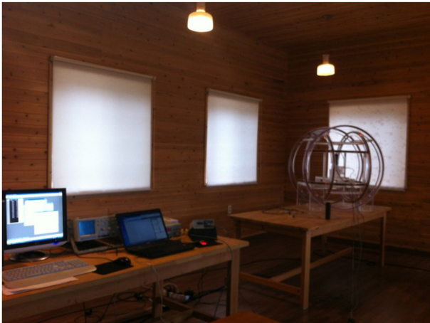
Fig. 3. (Color online) 3-axis Helmholtz coil system in side of non-magnetic laboratory for calibration of the magnetometer.
