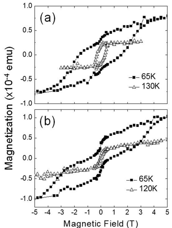
Fig. 4. Magnetization versus magnetic field curves of (a) as-grown and (b) post-growth annealed  $\text{CoMn}_2\text{O}_4/\text{Nb-STO}(100)$  thin films. The magnetic field was applied along the Nb-STO[100] in-plane direction.
