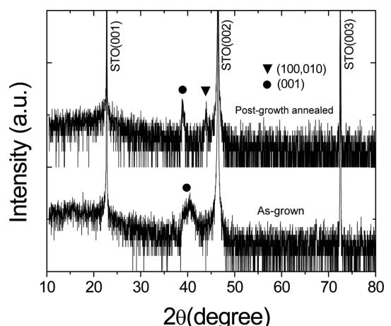
Fig. 1. XRD wide-2 scans for the as-grown and post-growth annealed  $\text{CoMn}_2\text{O}_4/\text{Nb}-\text{STO}(100)$  thin films.
