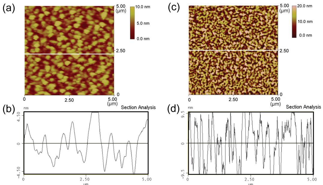
**Fig. 2.** (Color online) AFM images of (a) as-grown and (c) post-growth annealed CoMn<sub>2</sub>O<sub>4</sub>/SrTiO<sub>3</sub>(100) thin films. (c) and (d) show cross section profiles for each.
